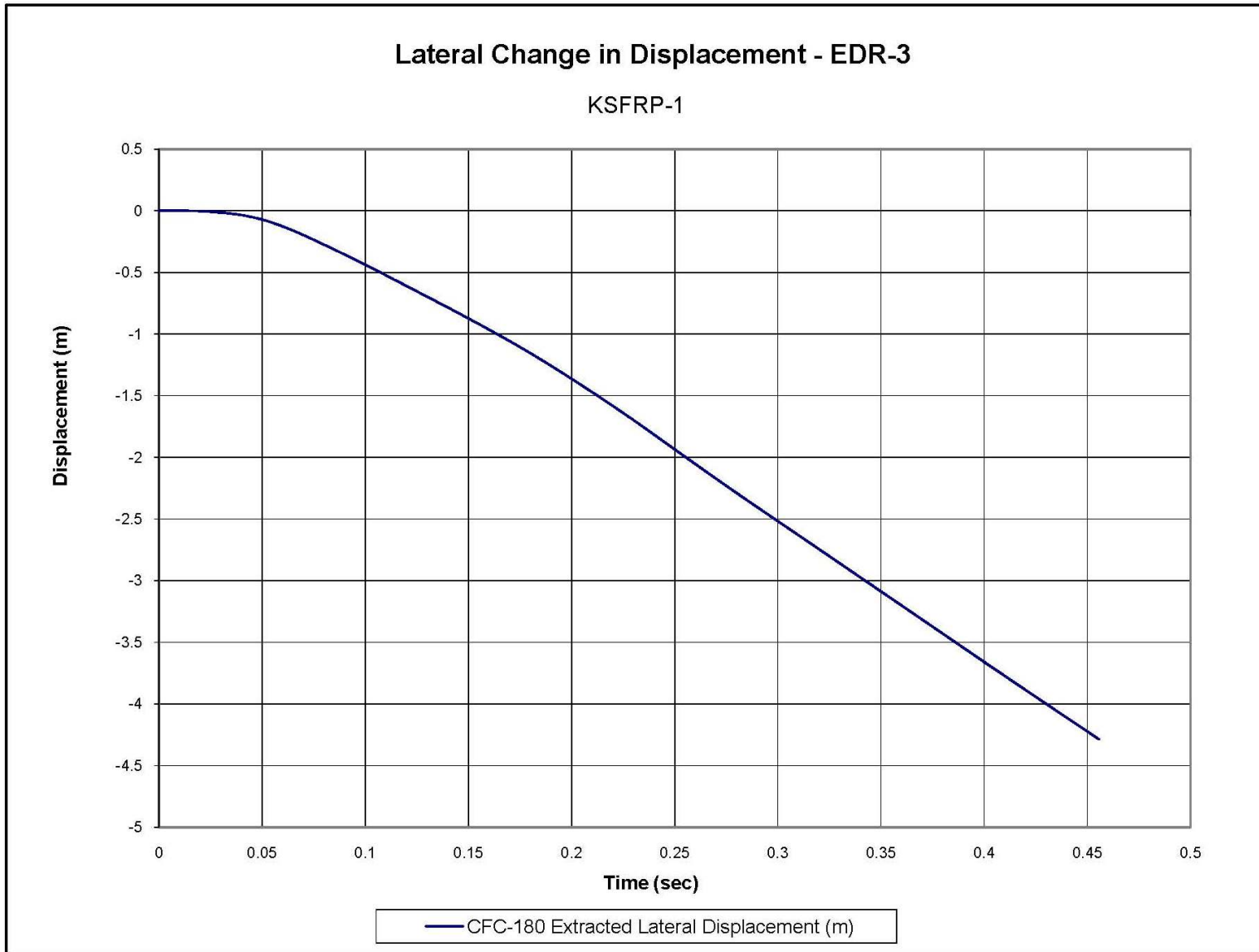
Figure D-6. Lateral Occupant Displacement (EDR-3), Test No. KSFRP-1
