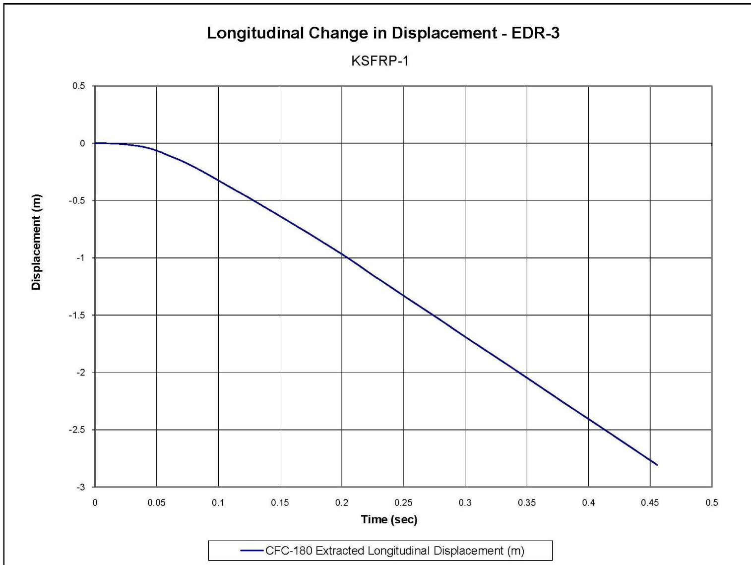
Figure D-3. Longitudinal Occupant Displacement (EDR-3), Test No. KSFRP-1
