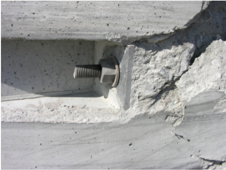
Figure 30. Joint Damage Between Barrier Nos. 2 and 3, Test No. KSFRP-1
