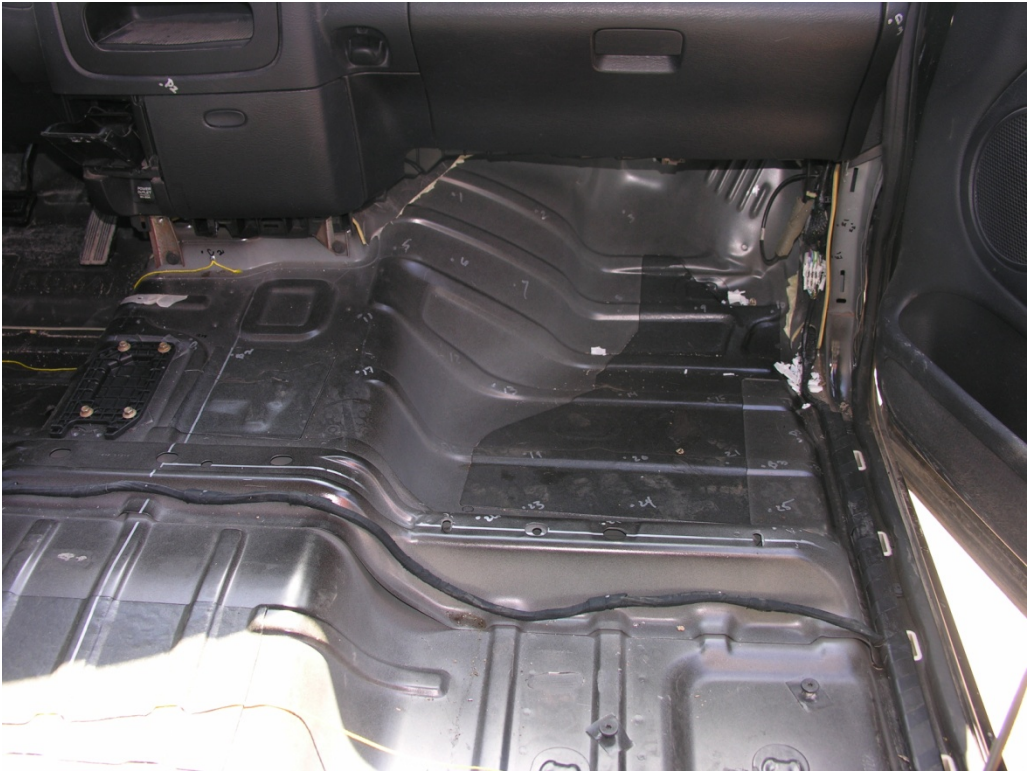
Figure 36. Interior Occupant Compartment Deformation, Test No. KSFRP-1
