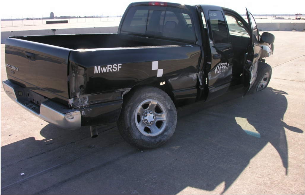
Figure 33. Vehicle Damage, Test No. KSFRP-1
